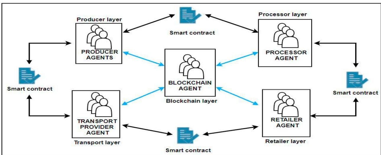
Fig. 4 - An example of an ordinary supply chain change utilizing blockchain technologies. Each layer sends data from its transactions to the blockchain. The layers that manage the articles also communicate with each other via smart contracts. These smart contracts enable the buying and selling of items.
